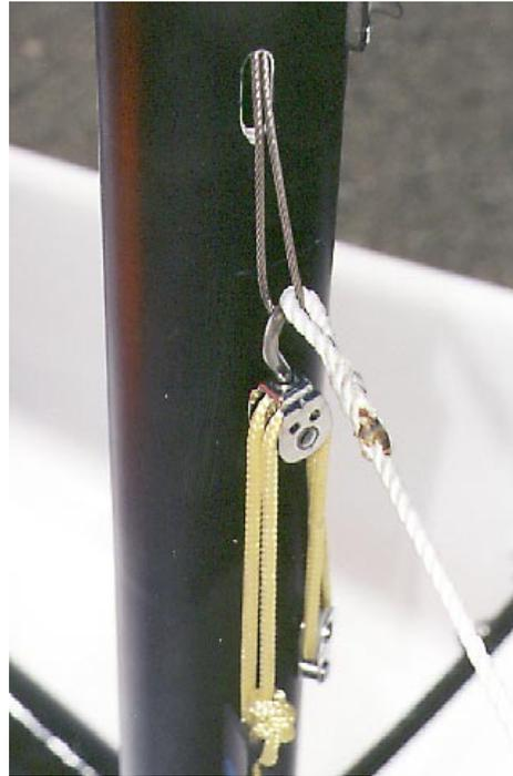
the wire loop to the adjustable rope purchase system. Don't over tension the jib halyard in light wind. If the leading edge of the jib looks stretched in light wind, it's too tight. Increase tension as the wind builds.
