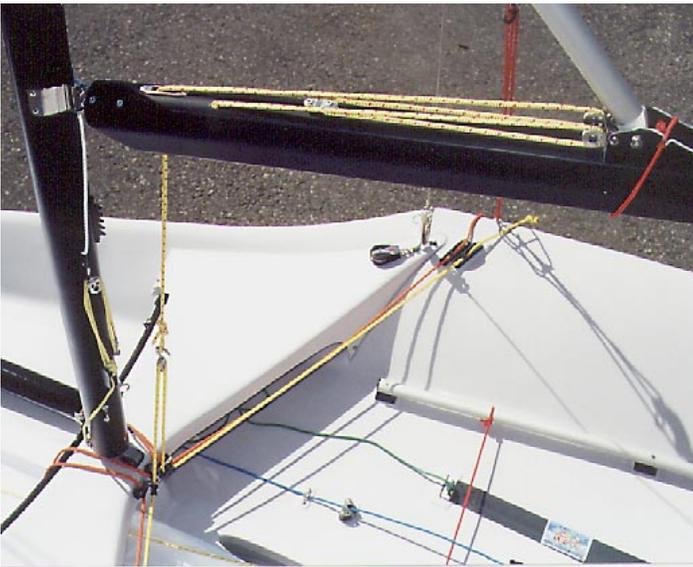
be free to slide. (Spray a little McLube on the felt under the shoe). The picture above shows the complete setup of the vang without the mainsail hoisted. The purchases on the boom are already rigged when shipped. Tie a loop in the end of line. The deck led part of the vang control attaches to this loop with the hook block.
