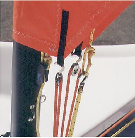
exiting from the bottom of the boom near the gooseneck. Zip up the main-sail sleeve.
