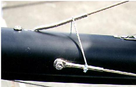
connect the forestay to the mast by first passing it underneath the small shock cord attached to the shrouds near the jib halyard sheave. The shock cord prevents the spinnaker halyard from getting caught in this area. The forestay should be taken off the mast while travelling as it sticks out beyond the mast step and has been known to fall out of the key slot. Undo the spinnaker halyard and **make sure there are stopper knots in both ends! Now!**
