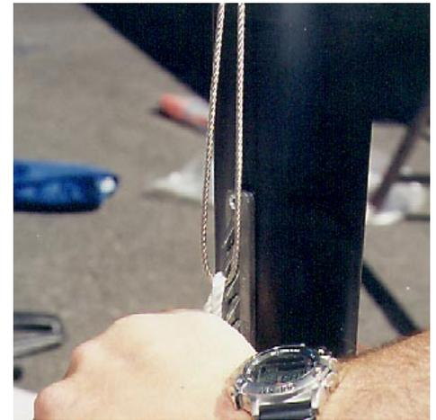
wire loop on to the teeth on the rack mounted on the side of the mast. Typically you will be on the first or second hook. Loop the clew tie-down over the end of the boom and attach the outhaul hook. (See earlier picture on p.2) Set the vang ram on the boom, and tuck all the halyard ends neatly inside the mainsail pocket.
