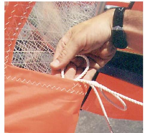
At this point you can attach the downhaul (Cunningham) hooks to the bottom of each side of the mainsail making sure that there are no twists in the purchase to allow for unencumbered adjustment. Also attach the vang adjustment hook to a bowline tied in the end of the vang shoe control line
