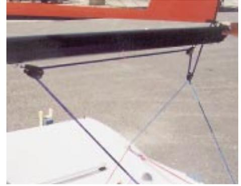
knot tied to the small saddle (deck strap). The final part passes through the block on the traveler and is tied off on the clew board (shown here being held by hand in the photo). The rules allow a shackle or quick release device for attachment to the clew.
