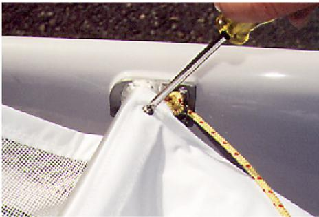
The first step is to lead the spinnaker halyard from where it exits the bottom of the mast straight down through an eye in the partner where it then passes forward through the cheek block mounted directly below on the side of the mast support. See below. It then goes towards the bow, **UNDER** both
