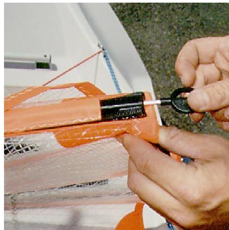
There is a key in a small pocket at the tack of the mainsail. Tension the battens with this key (counter clockwise) until they are just starting to stretch the pocket but not so much so that the sail is being heavily curved.
