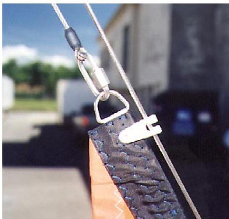
The jib clips directly onto the forestay, and the D ring in the tack is secured by a clevis pin and ring in the
