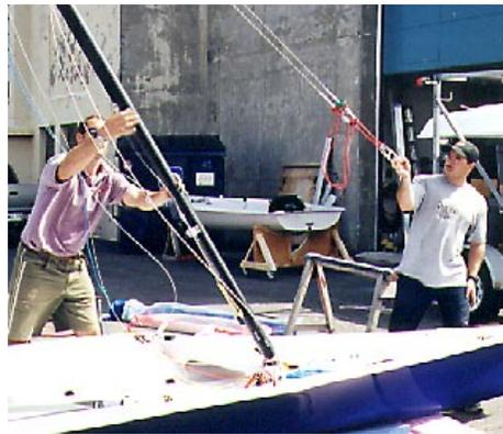
shrouds connected, make sure the trapeze wires are in an unobstructed position where they can help pull the mast upright as the person holding the tip walks it up beside the boat until out of reach.
